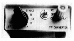
Converter front view. The power switch is a two-pole, three-position affair that switches the converter off and leaves the receiver operating as an independent unit. The converter weighs about 12 ounces (340 grams); current drain is 10 mA at 12 Vdc.
